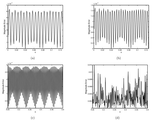
Fig. 4.4. The error distribution at the aperture of the empty cavity for  $k = 300\pi, 400\pi, 500\pi, 600\pi$  in (a), (b), (c) and (d) separately with  $1024 \times 1024$  meshes.
