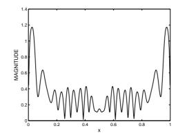
Fig. 4.5. Magnitude of the aperture field at normal incidence with homogeneous medium  $\varepsilon_r = 1.0$  when  $k_0 = 32\pi$ .
