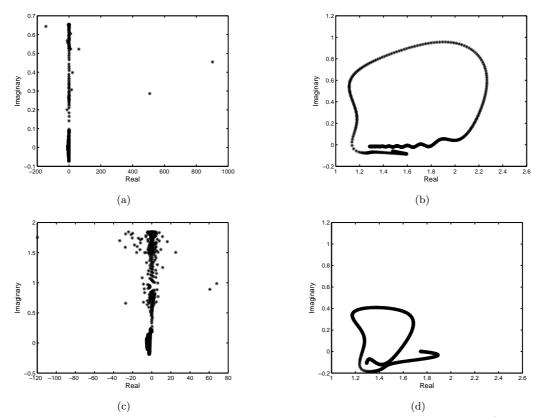
Fig. 4.2. The eigenvalues distribution of the unpreconditioned B and preconditioned  $M^{-1}B$  for the cavity filled with the medium of  $\varepsilon_r = 4 + i$  with  $1024 \times 1024$  meshes when  $k = 100\pi$  and  $300\pi$  separately in the TM case.
