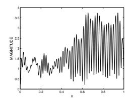
Fig. 4.6. Magnitude of the aperture field at  $\theta = \pi/4$  with homogeneous medium  $\varepsilon_r = 1.0$  when  $k_0 = 64\pi$ .
