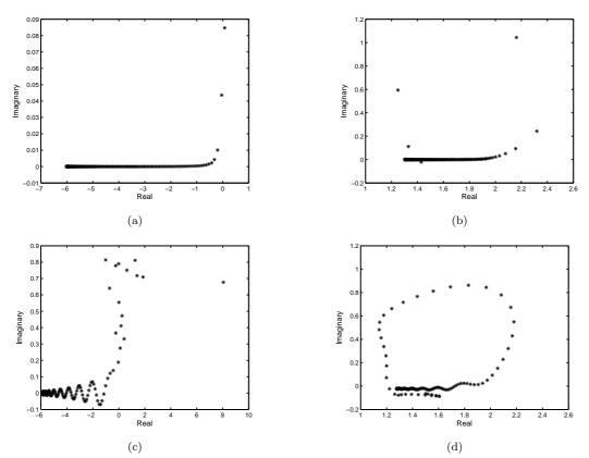
Fig. 4.1. The eigenvalues distribution of the unpreconditioned B and preconditioned  $M^{-1}B$  for the cavity filled with the medium of  $\varepsilon_r = 4 + i$  with  $128 \times 128$  meshes when  $k = 2\pi$  and  $16\pi$  separately in the TM case.
