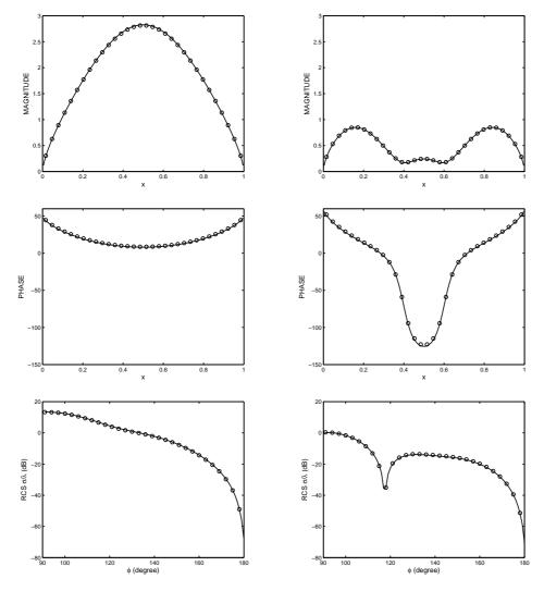
Fig. 4.7. The magnitude and phase of the aperture of electric field at normal incidence and the backscatter RCS for the empty cavity ( $\varepsilon_r = 1.0$ ) and the filled cavity ( $\varepsilon_r = 4.0 + i$ ) in the TM case when  $k_0 = 2\pi$ .
