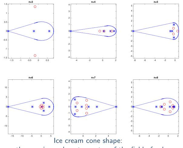
exactly one eigenvalue at a vertex of the field of values Solid blue curve is boundary of field of values of final computed ABlue asterisks are eigenvalues of final computed ASmall red circles are roots of final computed p
