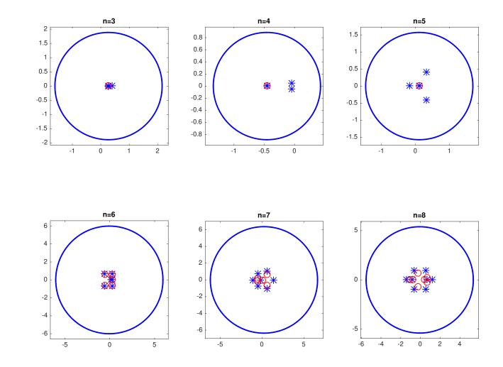
Solid blue curve is boundary of field of values of final computed A Blue asterisks are eigenvalues of final computed A Small red circles are roots of final computed p n = 3, 4, 5: two eigenvalues of A and one root of p nearly coincident 22 / 44
