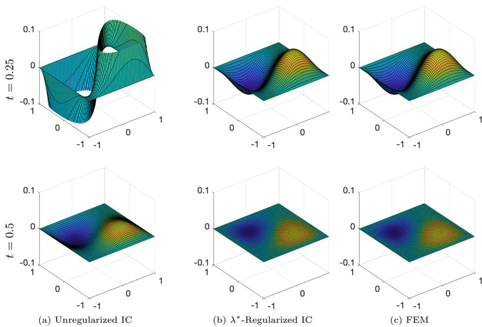
Figure 6: Example 5. Snapshots at time  $t = 0.25$  and  $0.5$  of numerical solutions for a heat equation obtained by (a) the method of lines with unregularized and (b)  $\lambda^*$ -regularized initial conditions (IC), and (c) finite element method.
