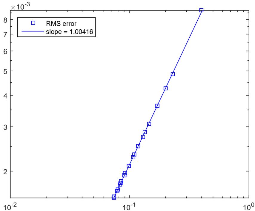
Figure 2: Convergence plot of diffusion on punch-in sphere.
